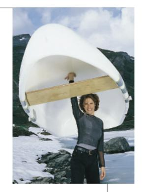
Traditional rubber dinghies are usually composed of tube-like elements. These trivial pneumatic structures give them a rather clumsy appearance, a high flow resistance and make them voluminous and space-consuming. On the other hand the elegant DINGHY, another demonstration model of a new technology, does not have any of these disadvantages.
