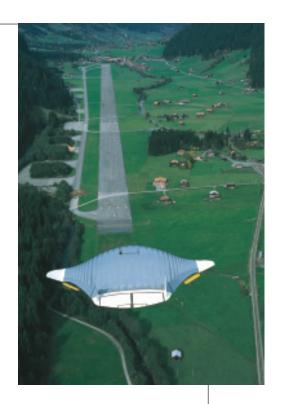
From 1995 through 2000, the STINGRAY, packed with sensor electronics, has completed over 300 test flights in Hradcany, Czech Republic, and St. Stephan, Bernese alps. In addition to aspects regarding aerodynamics and flight mechanics, the main focus was on analyzing the reaction of the pneumatic textile structure method to different forces. The STINGRAY was navigated by former airforce pilot Gion Bezzola.
