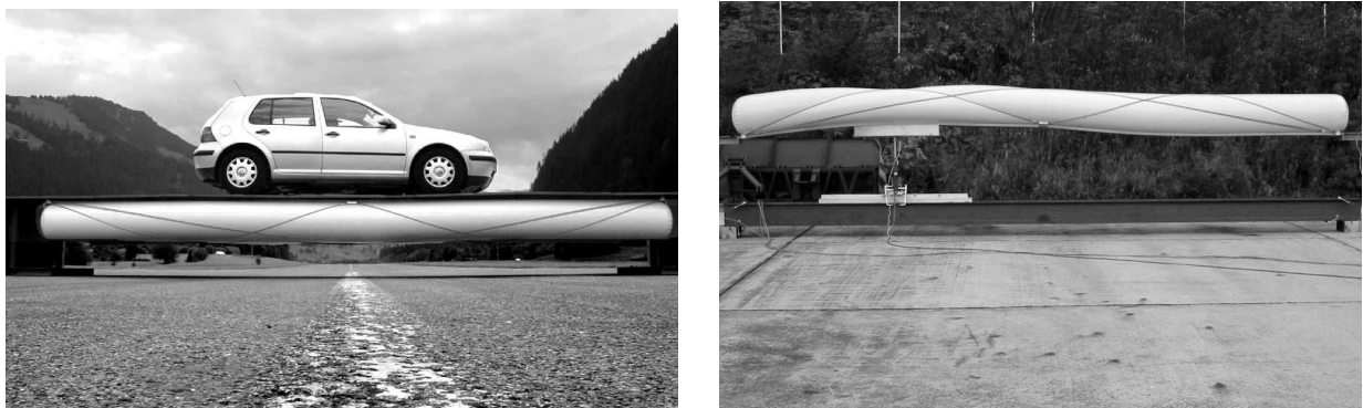
Fig. 4 Strong pneumatic structures with Tensairity: Tensairity demonstration bridge with 8 m span and 3.5 tons maximal load (left) and an ultimate load test of a Tensairity beam (right).
