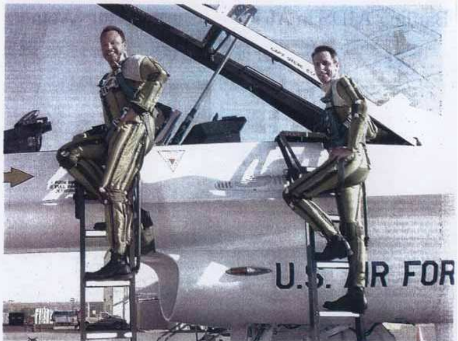
Lt. Col. Michael Sizoo, left, and Maj. Christian Ledet wear the Air Force's new antigravity suits, designed to counter the effects of rapid acceleration.
